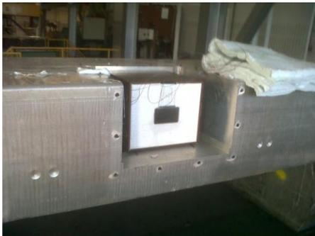
Figure 3. 'Hot Box' system being prepared on aluminium slab
