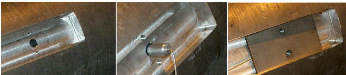
Figure 7. From left: slot machined in slab, thermocouple in bush inserted into slab, steel plate fitted to hold thermocouple in position
