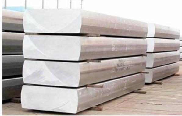
Figure 1. Aluminium slabs prior to rolling
