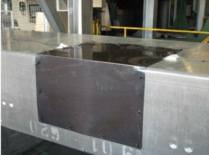
Figure 6. System mounted in slab with stainless steel cover to protect from high velocity air flow in furnace
