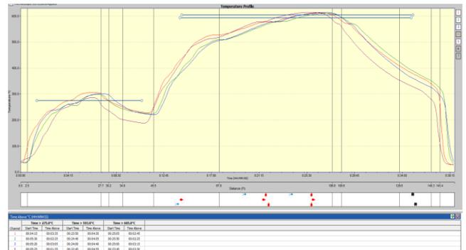
Typical profile obtained using a 'through furnace' temperature data logging system
