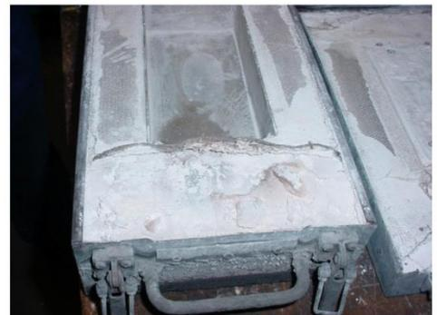
Acid attacks the cloth protecting the insulation
