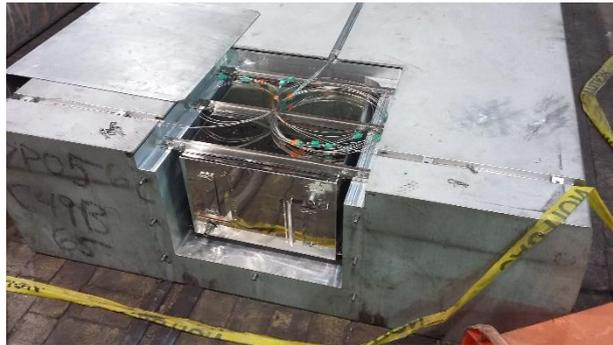
Fig 3: PhoenixTM System embedded in aluminium slab/Ingot - stainless steel cover to protect from high velocity air flow in furnace.
