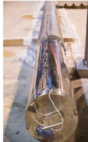
Fig 4: PhoenixTM Cylindrical Rotating Water barrier fixed to the aluminium log
