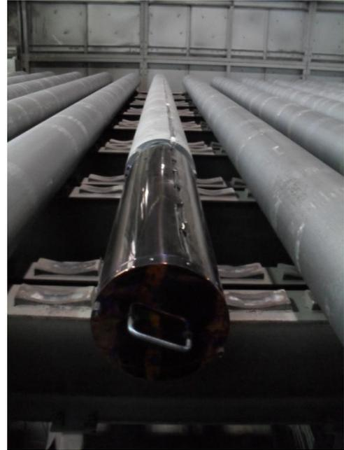
Figure 9 aluminium logs exit the furnace. The system is fixed to a shortened log, in which thermocouples are embedded.
