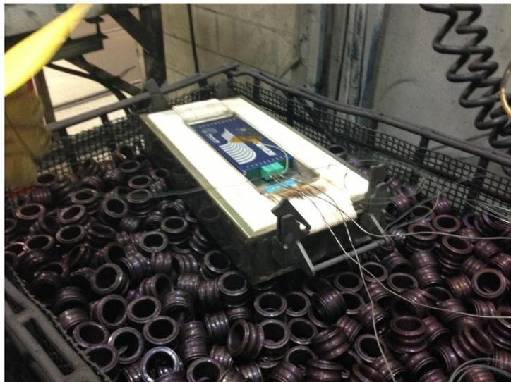
Figure 1 'Hot Box' system in product basket (shown open and with telemetry transmitter fitted)
