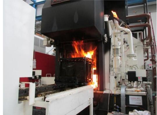
Figure 11 'Hot Box' system entering batch carburising furnace with oil quench
