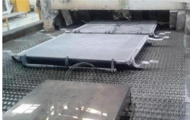
Figure 4 system entering CAB brazing furnace with product
