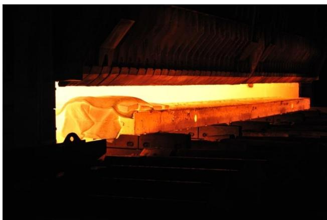
Figure 3 monitoring a steel slab being reheated prior to hot rolling.
