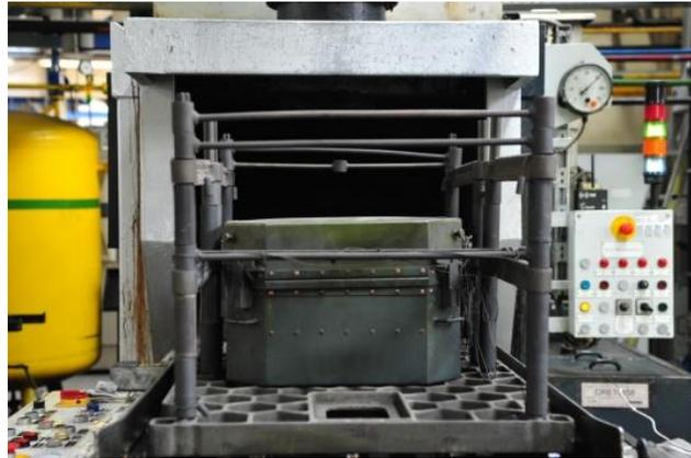
Figure 7 survey basket prepared on tray of pusher furnace
