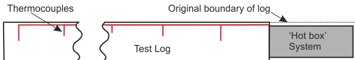
Figure 3 the monitoring system and thermocouples must not exceed the boundaries of the product
