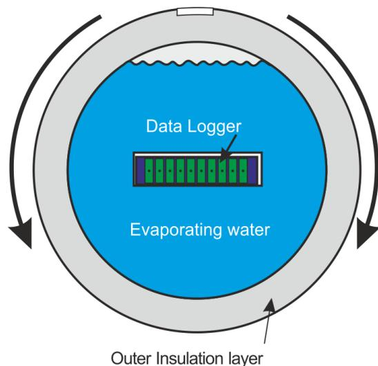
Figure 4 when fixed to the test log, the thermal barrier and data logger must rotate with the product
