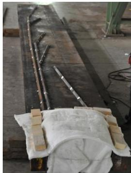
The test slab with thermocouples beneath the upturned angle iron protection. The data logging system is within the insulated package at the rear
