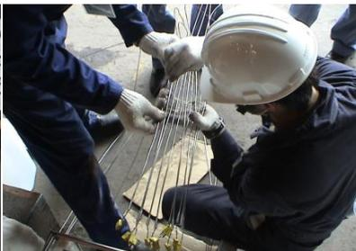
Data loggers which can accept up to twenty channels are now obtainable. But the number of thermocouples must be balanced against the difficulties of manipulating these on the test slab, and into the thermal protection
