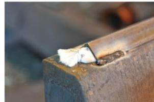
Compressed fibre insulation maintains a downward pressure on the thermocouple keeping it in contact with the bottom of the hole (where the measurement is required).
