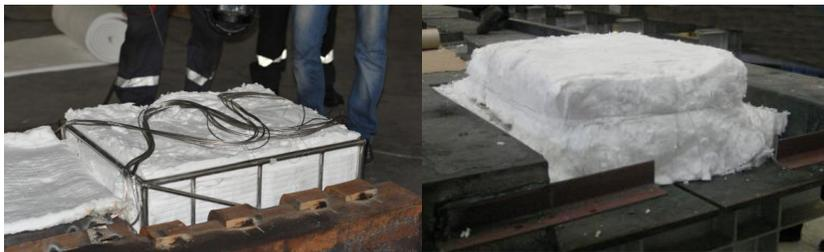
The excess length of thermocouples is carefully wound on top of the insulated thermal barrier and covered with extra insulating blanket to reduce heat.
