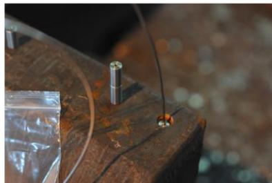
Steel ‘bushes’ guide the thermocouple down to its measurement point. These have heat transfer characteristics to the slab material
