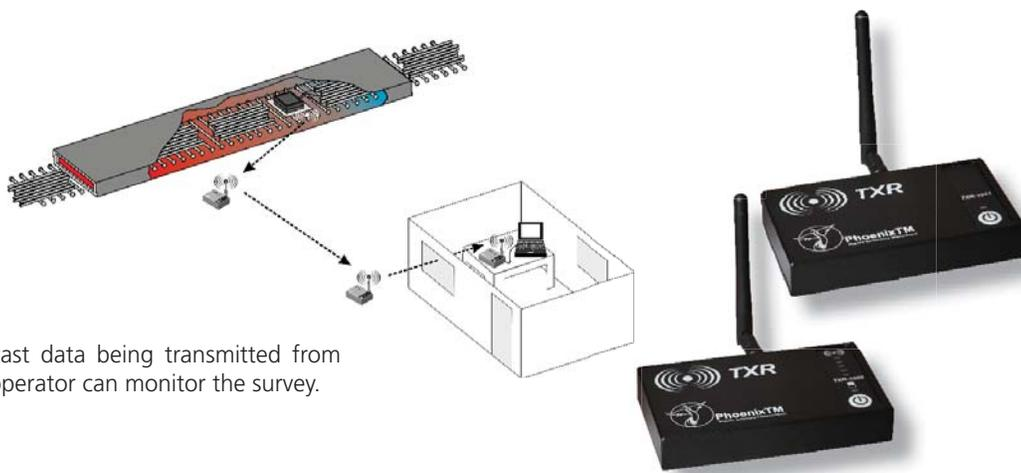
A series of routers can pick up and re-broadcast data being transmitted from within a furnace, to a remote office where the operator can monitor the survey.
