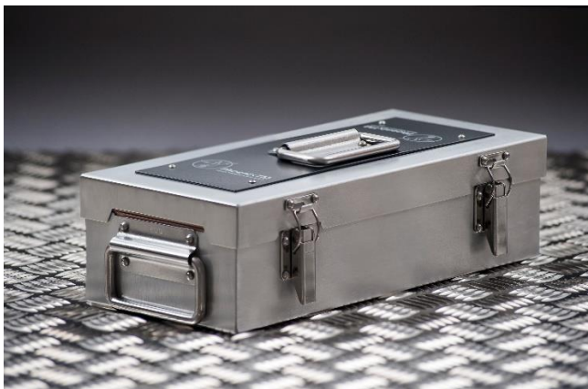
Figure 4: Aluminium, Silicone Free Finishing Thermal Barrier – (4.1) Mag Plate (4.2) Heatsink Thermal Protection @ 200 °C/392 °F (20 Channel Logger) TS04-XX (XX = Height mm) (TS04-60 0.8 hrs, TS04-113 3 hrs & TS04-135 4.8 hrs)
