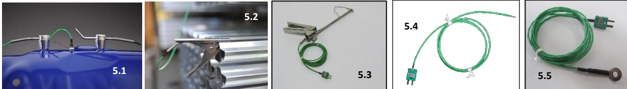
Figure 5: Thermocouple Range for Paint Applications (Surface and Air Options)
