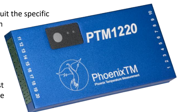
Fig 2: PhoenixTM PTM1220 20 Channel IP67 Datalogger
