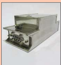
Fig.15: The 'Hump-back' evaporative thermal barrier with stepped profile to match the product and allow direct loading by robotic gripper into the furnace with test product.
