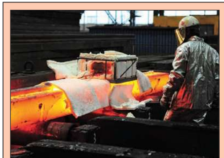
Fig. 4: PhoenixTM profile system post reheat furnace. Thermal barrier (TS07-300-3, 3.2 hours protection at 1300°C) loaded on cast steel beam blank reheated prior to rolling into structural metalwork for buildings/skyscrapers. The PhoenixTM 1220 data logger, at the core of the system, stores data measured by the thermocouples inserted into blank at varying depths along its length.
