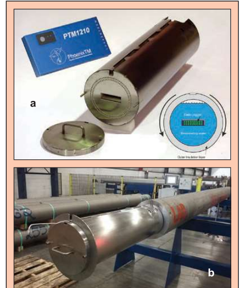
Fig. 12: Cylindrical evaporative thermal barrier technology for use in walking-beam aluminium log homogenisation furnace: (a) cylindrical barrier design and water tank schematic; (b) barrier secured to test aluminium log.
