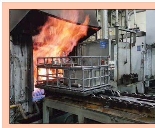
Fig. 2: 'Thru-process' temperature monitoring system loaded in a charge basket, travelling into and through a continuous gas carburising furnace, and typical resulting thermal profile.
