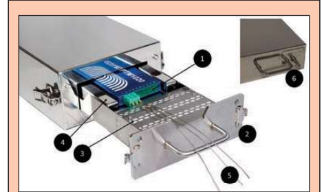
Fig. 13: CAB brazing thermal barrier design: (1) data logger (6 or 10 channels); (2) front-loading logger tray with encapsulated insulation; (3) thermal breaks reduce conduction to data logger; (4) heat sink provides additional thermal protection; (5) mineral-insulated thermocouples attached to radiator fin; (6) nitrogen feed nozzle for insulation purge.
