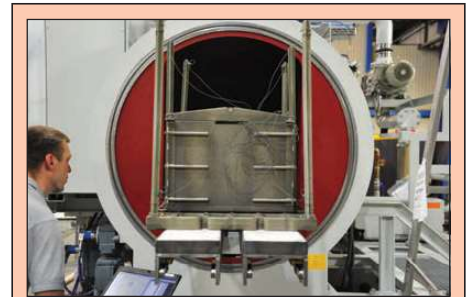
Fig. 7: Thermal barrier fitted with quench deflector being loaded into LPC batch furnace with TUS frame as part of temperature uniformity survey.
