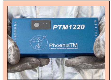
Fig. 1: Typical temperature data logger (up to 20 thermocouple inputs) used in a 'thru-process' system. Protected by a thermal barrier, it travels through the furnace with the product being monitored. Data are stored in memory for download post run or are transmitted live from the furnace using a RF telemetry option.
