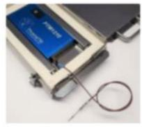
Employing the thruprocess temperature monitoring principle provides the food technologist with a complete temperature profile of the cook process from start to finish.
