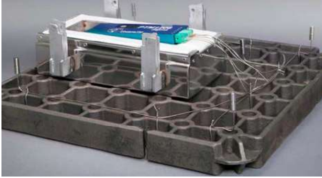
Figure 6. (left) Low profile TUS system (TS02-128-1 thermal barrier six channel Sigma data logger) designed with TUS Thermal barrier shown with optional low profile gas quench deflector. (right) Thermal barrier shown with optional low profile gas quench deflector. (Source: PhoenixTM)
