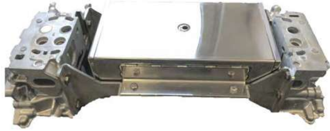
Figure 7. (left) Robot loading of combined thru-process system with engine block into BSN rotary T6 furnace. The thermal barrier is designed with a combination of thermal insulation technology capable of fitting in the engine block cavity. (right) Thermal barrier mounted within engine block assembly. (Source: BSN Thermprozessechnik GmbH)
