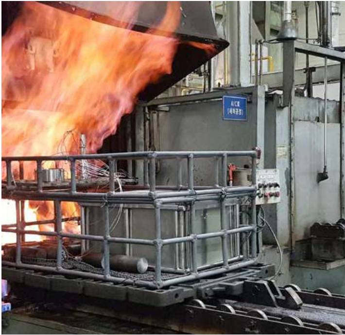
Figures 4. Phoenix TM thru-process temperature profiling system monitoring the core temperature of automotive parts in a traditional sealed gas carburizing furnace with integral oil quench. (left) System entering carburizing furnace in product basket. (right) Thermal barrier showing outer structural frame and sacrificial insulation blocks protecting inner sealed thermal barrier housing the data logger. (Source: Phoenix TM )
