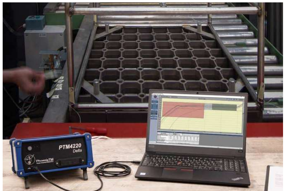
Figure 1. Typical TUS survey set-up for a static batch furnace. PhoenixTM PTM4220 External data logger connected directly to a 9 point TUS frame used to measure the temperature uniformity over the volumetric working volume of the furnace. (Source: PhoenixTM)
