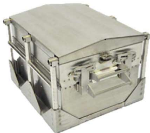
Figures 5. (left) Thermal barrier being loaded into LPC batch furnace with TUS frame as part of temperature uniformity survey. (right) Thermal barrier shown with independent quench deflector providing protection during the high pressure gas quench. (Source: PhoenixTM)
