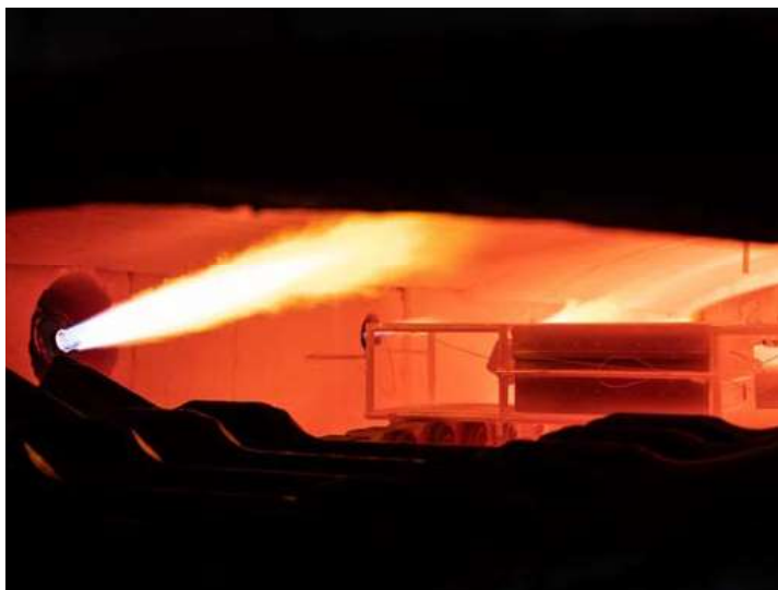
Figures 3. Temperature uniformity survey of a continuous furnace using the plane method applying the PhoenixTM thru-process monitoring system. The data logger travels protected in a thermal barrier mounted on the TUS frame performing a safe TUS at four points across the width, which is impossible with trailing thermocouples. (Source: Raba Axle, Győr, Hungary)
