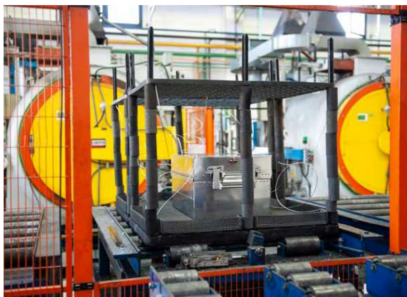
Figures 5. (left) Thermal barrier being loaded into LPC batch furnace with TUS frame as part of temperature uniformity survey. (right) Thermal barrier shown with independent quench deflector providing protection during the high pressure gas quench. (Source: PhoenixTM)
