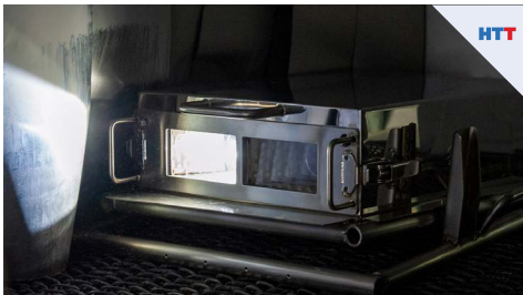
Figure 5.1. High temperature thermal barrier for aluminum brazing system protecting camera and torches through CAB furnace
