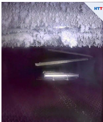
Figure 5.3. Identification of flux debris at back end of muffle furnace prompting scheduling of clean down operation
