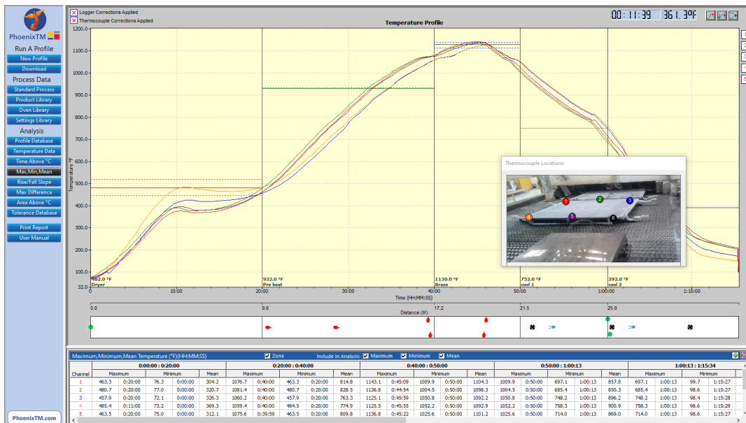
Figure 3. Typical temperature profile recorded for an aluminum CAB brazing line giving a complete temperature history for a brazed radiator at different product locations. 1
