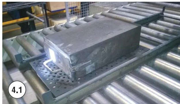
Fig. 4. Phoenix™ optical-profiling system being used in a conveyORIZED aluminum brazing furnace
