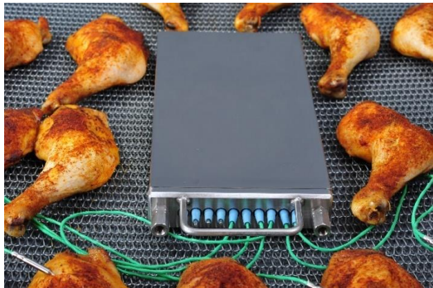
Fig 1: PhoenixTM food thru-process temperature profiling system monitoring chicken cook in linear conveyerized oven.
