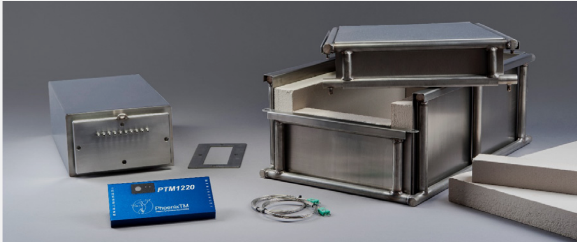
Fig. 13: Components of the PhoenixTM measuring system used [18]
