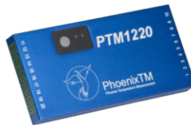
Fig 3: PhoenixTM PTM1220 20 Channel IP67 data logger comes calibrated to UKAS ISO/IEC17025 as an option with an onboard calibration data file allowing direct data logger correction factors to be applied automatically to TUS data.
