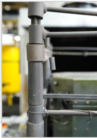
Photograph of thermocouple secured to TUS frame with heat sink (6.3).
