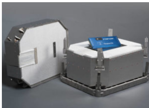
Fig 4: "Octagonal" thermal barrier fitted to product/survey tray.
