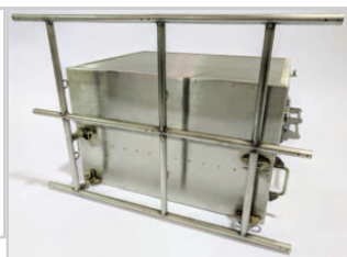
Fig. 8.2. Photograph of barrier designed with mounted thermocouple fixing rig for TUS monitoring, employing the plane method.
