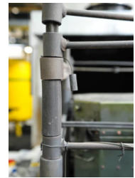
Photograph of thermocouple secured to TUS frame with heat sink (6.3).
