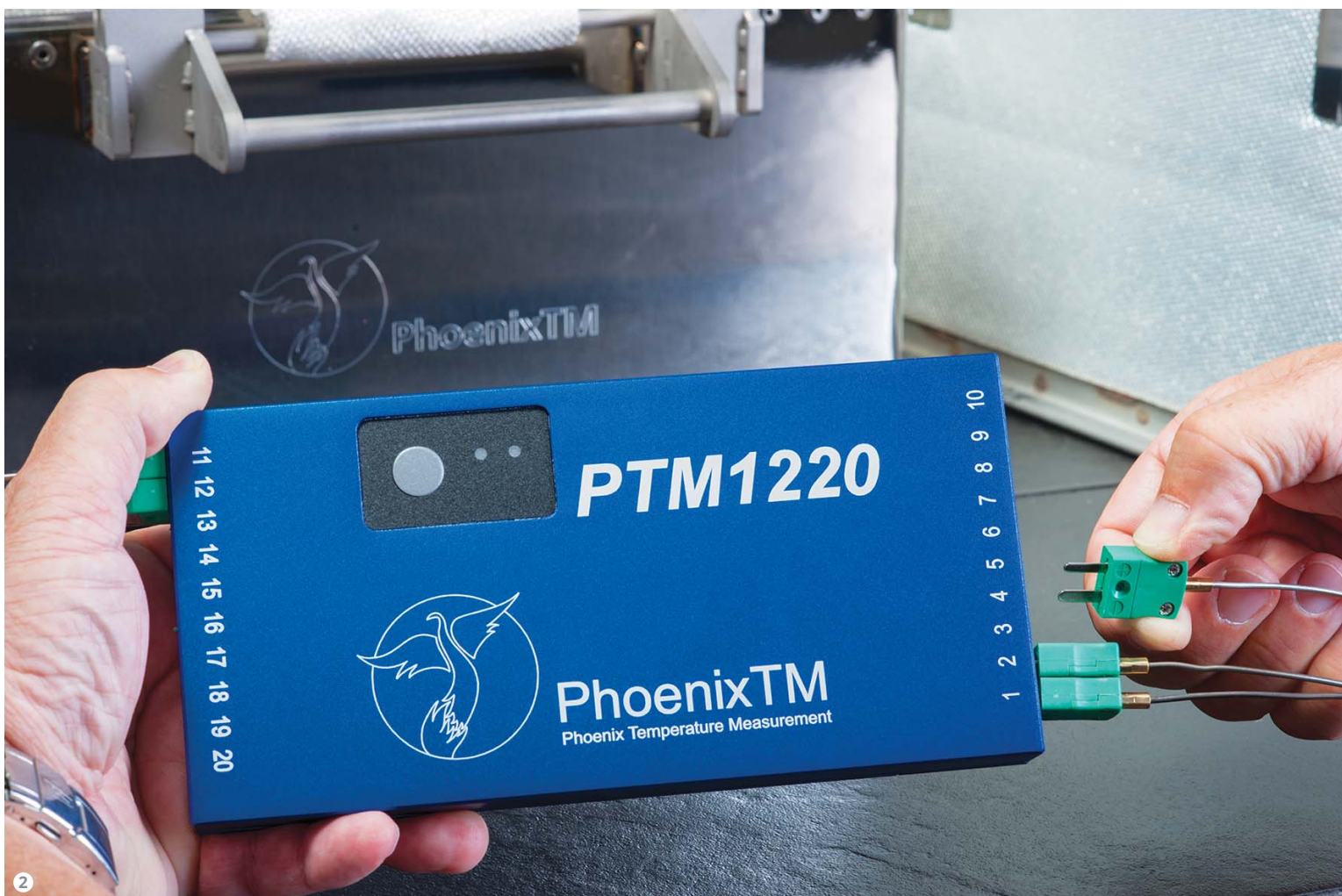
Figure 2: The new model PTM1-200-LT data logger with a maximum operating temperature of 80 °C is available in either 6, 10, or 20-channel versions.
