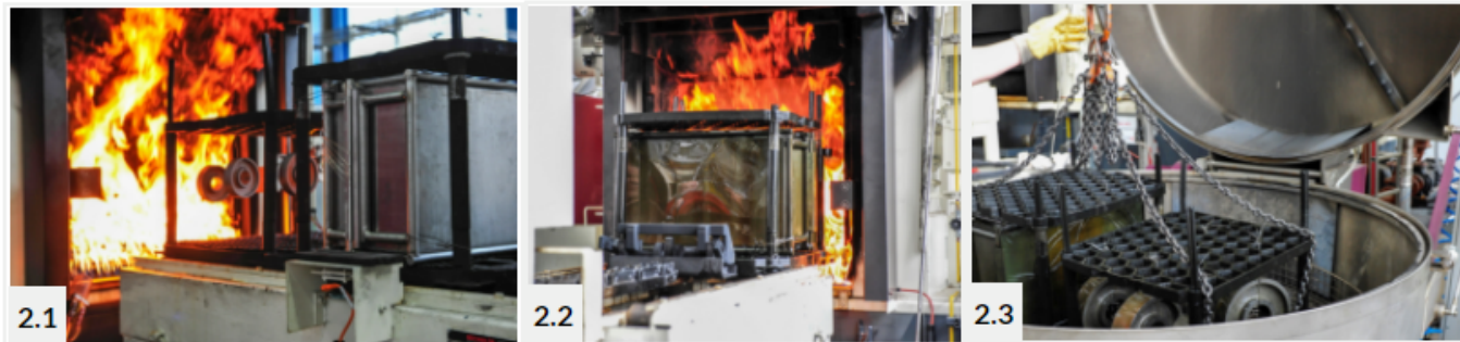
Fig. 2. A thru-process temperature monitoring system for use in a sealed carburizing furnace with integral oil quench. (2.1) Monitoring system entering furnace with thermocouple fixed to automotive gears, product test pieces; (2.2) System exiting oil quench tank; (2.3) System inserted into wash tank with product basket
