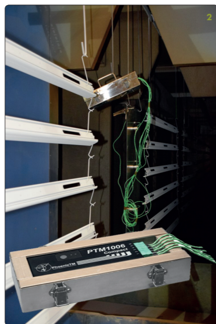
Figure 2: PhoenixTM Compact System travelling through a Powder Coating Oven with Aluminium Extrusion Products. (Insert Data logger Installed in thermal barrier shown in main image)
