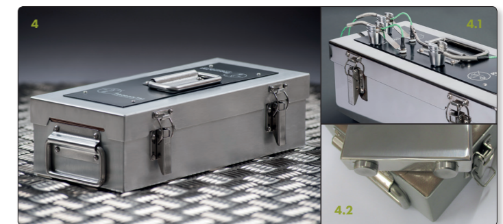
Figure 4: Aluminium, Silicone Free Finishing Thermal Barrier – (4.1) Mag Plate (4.2) Heatsink. Thermal Protection @ 200 °C (20 Channel Logger) TS04-XX (XX = Height mm) (TS04-60 0.8 hrs, TS04-113 3 hrs & TS04-135 4.8 hrs
