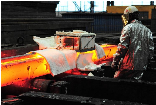
Fig 4: PhoenixTM Profile system post reheat furnace. Thermal barrier (TS07-300-3 3.2 hrs protection at 1300 °C / 2372 °F) loaded on cast steel beam blank reheated prior to rolling into structural metal work for buildings/skyscrapers. The PhoenixTM 1220 data logger at the core of the system stores data measured by the thermocouples inserted into blank at varying depths along its length.
