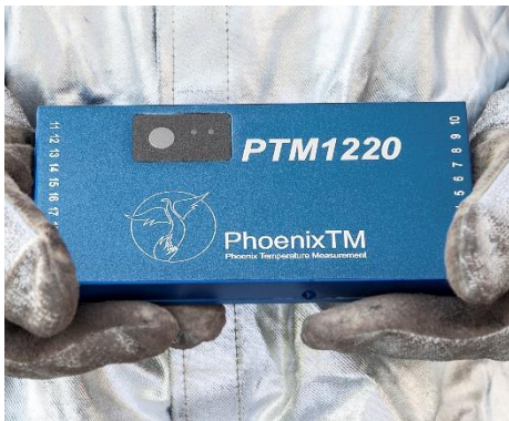
Fig 1: Typical temperature data logger (up to 20 thermocouple inputs) used in a 'Thru-process' system. Protected by a thermal barrier it travels through the furnace with the product being monitored. Data is stored in memory for download post run or is transmitted live from the furnace using a RF Telemetry option.
