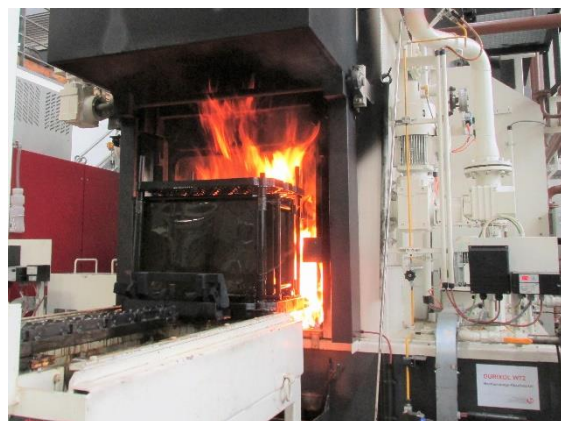
Fig 11: 'Thru-process' temperature monitoring system for use in sealed carburizing furnace with integral oil quench – (11.1) Barrier Construction (11.2) System in use in Sealed Gas Carburizing Furnace
