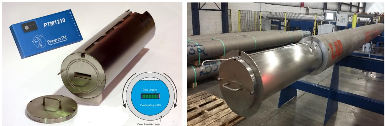
Fig 12: Cylindrical evaporative thermal barrier technology for use in walking beam aluminium log homogenisation furnace (12.1) Cylindrical barrier design and water tank schematic (12.2) Barrier secured to test aluminium log.
