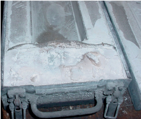
Fig 3. Damage to a conventional Thermal barrier design from flux materials reacting with moisture to form corrosive HF
