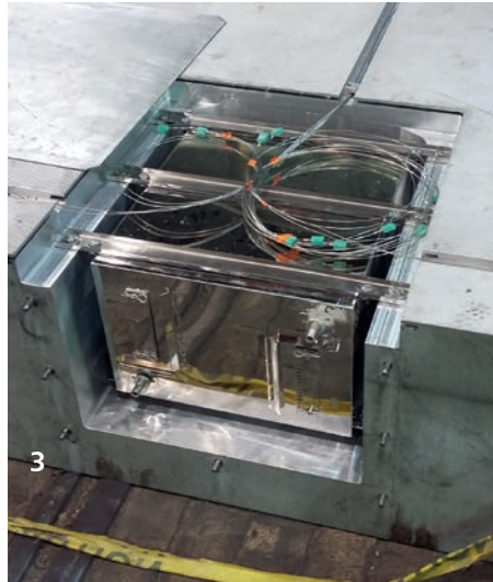
Fig 3. PhoenixTM System embedded in aluminium slab/ Ingot - stainless steel cover to protect from high velocity air flow in furnace
