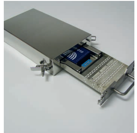
Fig 7. Unique Phoenix TM CAB Brazing System Design with contamination free profiling capability
