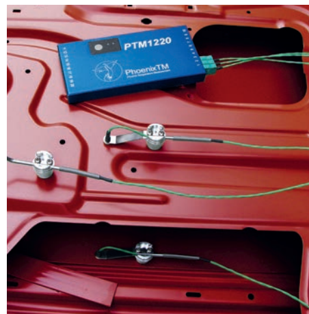
Fig 8. Phoenix TM finishing system showing PTM1220 20 channel logger with traditional magnetic thermocouples used on steel body shells. New aluminium clamp probe used on car bodies with aluminium sections (door skin, roof or hood).
