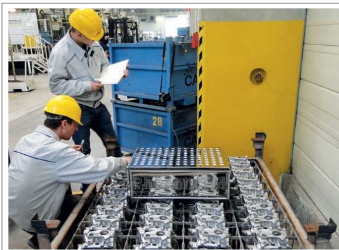
Fig 5. PhoenixTM HTS06 Solution Reheat System and Temperature Profile Trace collected from system
