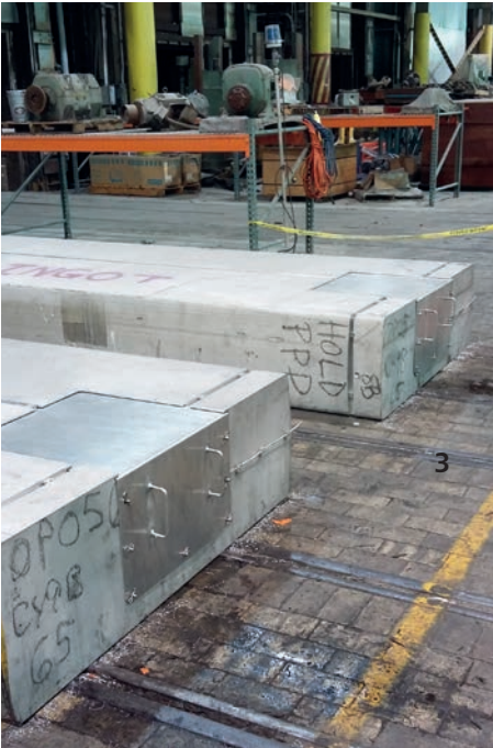
Fig 3. PhoenixTM System embedded in aluminium slab/ Ingot - stainless steel cover to protect from high velocity air flow in furnace
