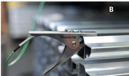
Fig 9: (A) PhoenixTM Compact Finishing System showing PTM1006 6 channel logger and (B) Clamp probe fixed to an aluminium extrusion (C) Phoenix TS01 system in Batch Age Hardening Oven
