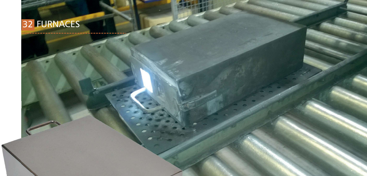
Fig 2. PhoenixTM Optical profiling 'Optic' System - High Temperature Thermal barrier used in the CAB brazing furnace protecting the video camera and dual torches
