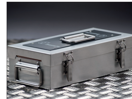
Fig 3. Aluminium, Silicone Free Finishing Thermal Barrier – (3.1) Enclosed Barrier (3.2) Heatsink Thermal Protection @ 200°C → TS04-XX (XX = Height mm) (TS04-60 0.8 hrs, TS04-113 3 hrs & TS04-135 4.8 hrs)
