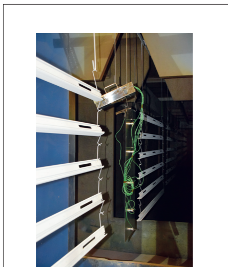
Fig 1. PhoenixTM Compact System travelling through a Powder Coating Oven monitoring Aluminium Extrusions
