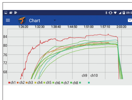
Fig 5. Thermal View Mobile software running on an Android smart phone allowing remote reset or download of the logger
