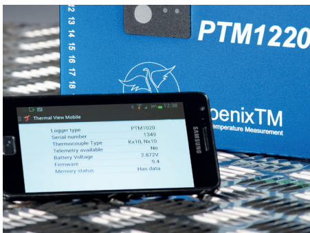
Fig 5. Thermal View Mobile software running on an Android smart phone allowing remote reset or download of the logger
