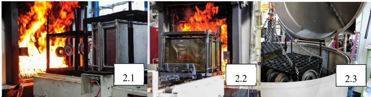
Figure 2: ‘Thru-process’ temperature monitoring system for use in a sealed carburising furnace with integral oil quench – (2.1) Monitoring system entering furnace with thermocouple fixed to automotive gears, product test pieces. (2.2) System exiting oil quench tank. (2.3) System inserted into wash tank with product basket
