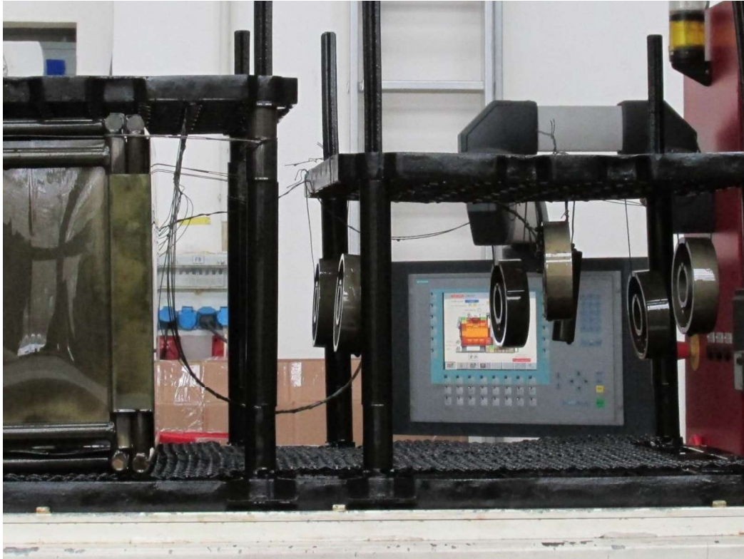
Figure 5: ‘Thru-process’ temperature monitoring system configured with test gear main bodies with thermocouples located at different locations on the gear body
