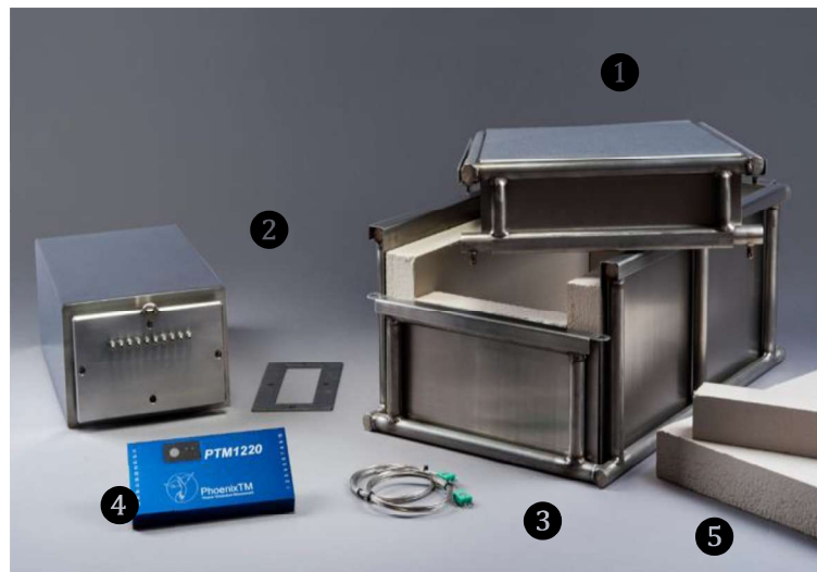
Figure 3: ‘Thru-process’ temperature monitoring system oil quench compatible thermal barrier design 1. Robust outer structural frame keeping insulation and inner barrier secure; 2. Internal thermal barrier – completely sealed with integral microporous insulation protecting data logger; 3. Mineral insulated thermocouples sealed in internal thermal barrier with oil tight compression fittings; 4. Multi-channel high temperature data logger; 5. Sacrificial insulation blocks replaced after each run
