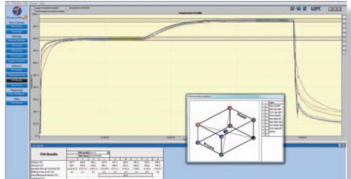
Comprehensive analysis tools are located on the left side of the screen for single click analysis and report generation. Data import and export in both .csv and PhoenixTM formats are available allowing electronic transfer of process data.
