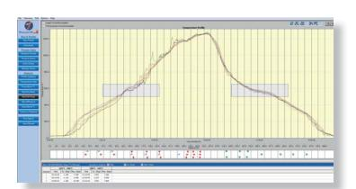
The temperature profile is displayed in the graphics window of the Thermal View software. Thermocouple profiles can be switched on or off individually and you can zoom in for more detailed analysis.
