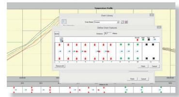
Comprehensive analysis tools are located on the left side of the screen for single click analysis and report generation. Data import and export in both .csv and PhoenixTM formats are available allowing electronic transfer of process data. User defined kiln zones and kiln features to support profile analysis.
