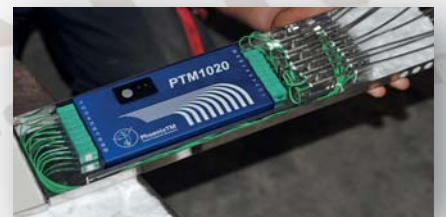
Integrated logger tray with thermocouple clamps for ease of data logger installation and removal
