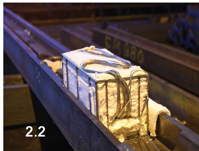
Fig 2: (2.1) Phoenix TM Profiling system showing typical thermal barrier design (thermal blanket insulated water tank) and data logger held in insertion tray. (2.2) System pre-run installed on steel blank. (2.3) System post reheat furnace. Thermal barrier (TS07-300-3 provides 3.2 hrs protection at 1300 °C / 2372 °F) loaded on cast steel beam blank reheated prior to rolling into structural metal work for buildings/skyscrapers. The Phoenix TM 1220 data logger at the core of the system stores data measured by the thermocouples inserted into the steel blank at varying depths along its length.
