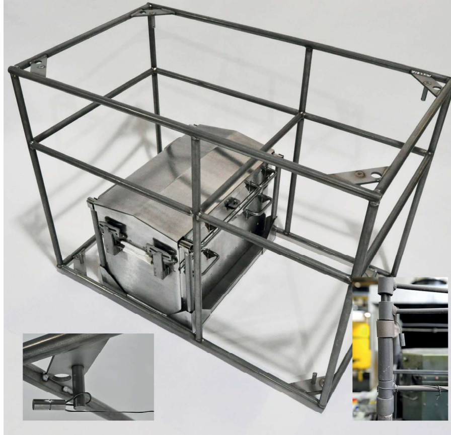
Figure 5: Phoenix™ Thru-process TUS system installed in Volumetric TUS Frame. Thermocouples mounted on fixed mounts at the eight vertices of the frame and centre point as shown with heat sink fixed to sensor hot junction.
